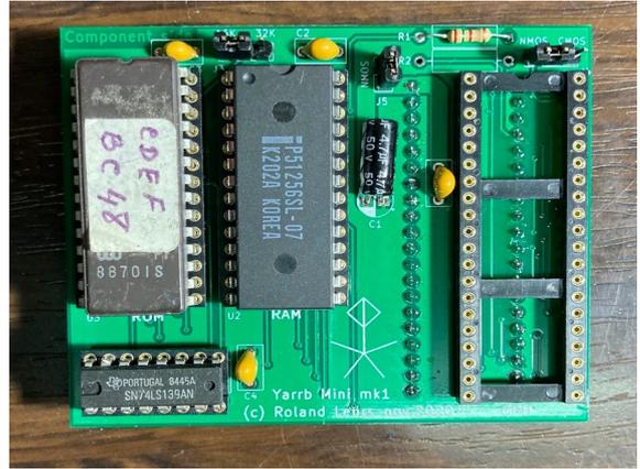
The Yarrb Mini board is a simple memory expansion board with 16K ROM (C-D-E-F blocks) and 32K RAM (#0000 – #7FFF). This board is designed for usage in an unexpanded Atom that does not use any external I/O expansions.
